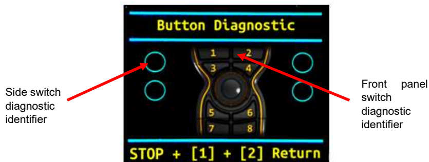
Figure 7. Button Diagnostic page on Transmitter
